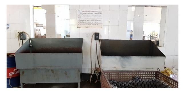
Oiling is one of the important process for heat treatment to the finish good. We provide oiling machine to oil the material with standard oil.
