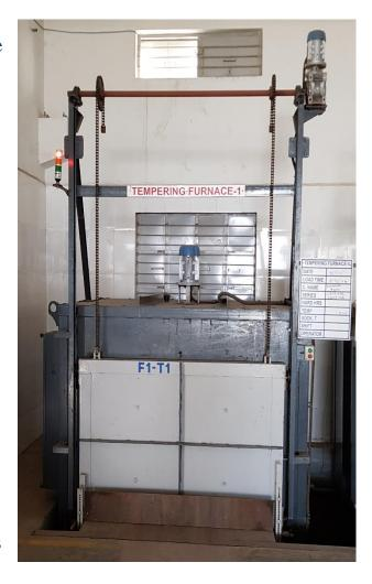
We provide tempering by electric resistance heating for uniform distribution of temperature with specific time. Our tempering furnace capacity up to 450°c
