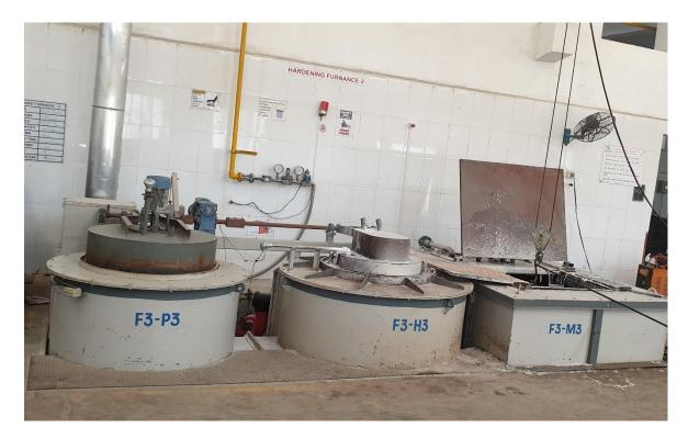
Preheating Furnace is provided with centrifugal air circulating fan for uniform preheating of material before immersed to saltbath.
