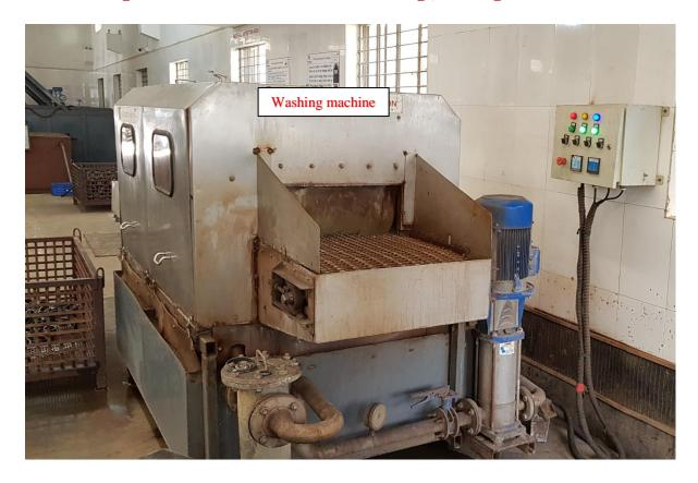
After the salt-bath heattreatment process washing is necessary of cleaning of material . we introduce Double chamber Conveyor type Automatic washing machine for this purpose instead of conventional washing method . High pressure water nozzles 120 NOS is fitted in chamber of machine that remove salt or any dirt from the material and its groove .
