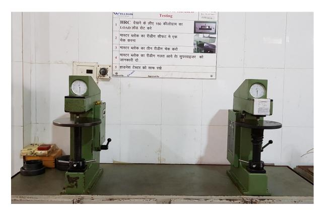
Hardness testing is heart of heat treatment process . We are using Saroj Made Rockwell hardness tester . We measure hardness of 10% of material at each batch of hardening . also hardness tester is calibrated by master block daily in time interval . We also send hardness report to the customer per batch .
